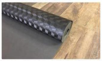
NOTE: When installing PHD for LVT in lower ground floors like basements or areas where a moisture barrier is required, spread out the underlayment 1"- 2" up the walls. New concrete should cure for 60-90 days minimum before installing. Check for excessive dampness before installation and refer to the flooring manufacturer's recommendations.
